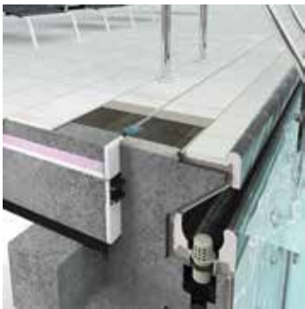
Large overflow channel with handhold-piece.
